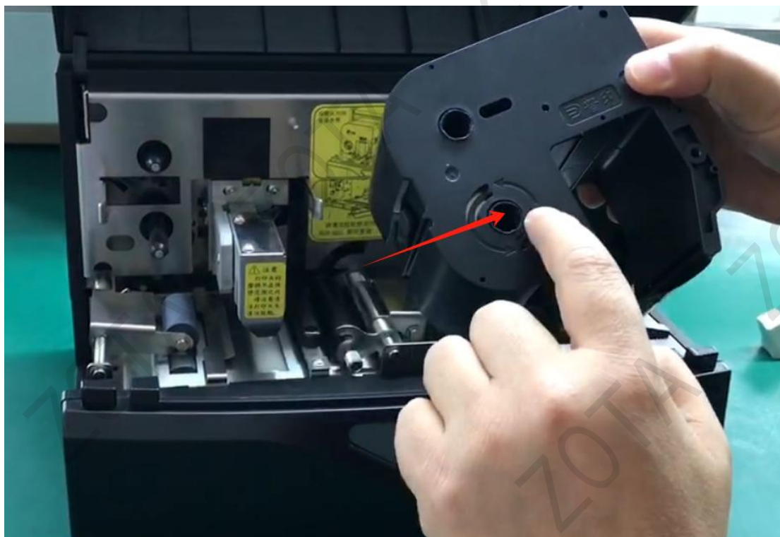
将色带沿金属卡槽位置平整推入 Push the ribbon flatly along the metal slot
